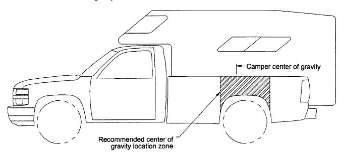
Any accessories or other equipment added to this vehicle after final date of manufacture must be weighed or have their weight determined, and the weight deducted from the prescribed Cargo Weight Rating (CWR) of this vehicle. This may decrease the permissible longitudinal zone of the center of gravity for this vehicle.
